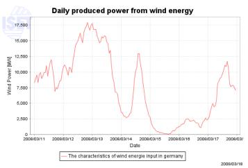
The output from even a large fleet of wind turbines (such as they have in Germany) can be very variable:
